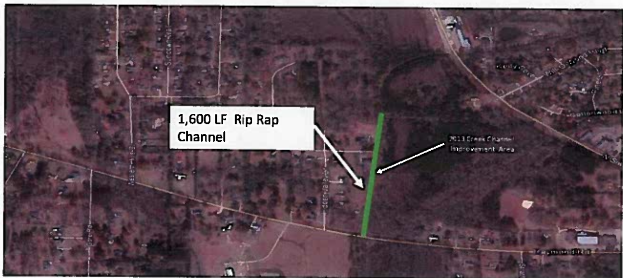
FIGURE 17 – 1 BIG CREEK BASIN NEAR TERM PROTECTION MEASURES HIDDEN VALLEY LANE CHANNEL RESTORATION PROJECT
