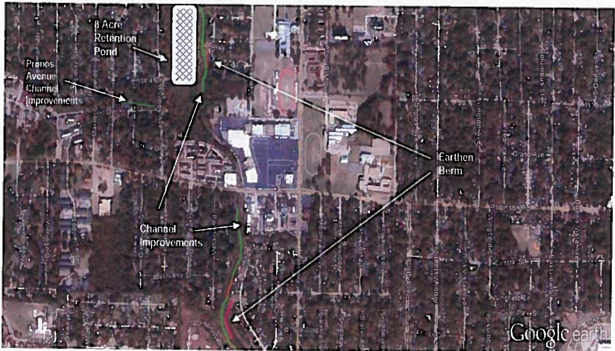
FIGURE 8 – 2 LYNCH CREEK BASIN IMMEDIATE MITIGATION MEASURES CASA GRANDE - HEMMINGWAY CIRCLE CHANNEL IMPROVEMENTS
